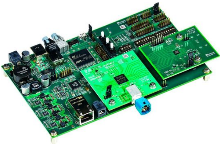
Fig. 4: With this modular developer platform, the APiX3-Link can be integrated into an existing system environment and evaluated. The video interface – such as DisplayPort on the Tx and DisplayPort, DSI or LVDS / oLDI on the Rx side – can be selected via piggyback boards. (Bild: Inova Semiconductors)
