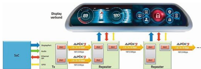
Fig. 2: Displays can be cascaded easily with the APIX3 repeater. Only one cable leads from the head unit to the display cluster; multiple image contents can be transported simultaneously via DisplayPort and APIX3. A significant saving in weight and costs.
