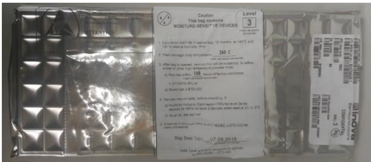
Figure 5 ESD protective dry bag for a single tray
